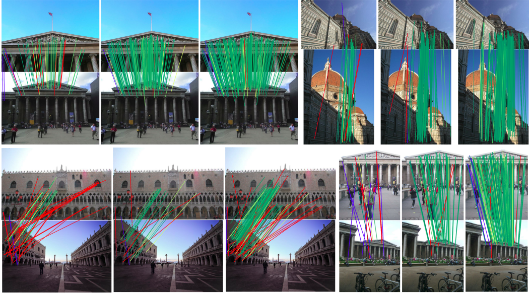
Figure 3: Matches Visualization. We visualize the matches produced by Superpoint (left), Upright RootSIFT (middle), and our method (right) for four stereo pairs in the test set of Phototourism dataset. Matches are coloured red to green, according to their reprojection error (high to low).
